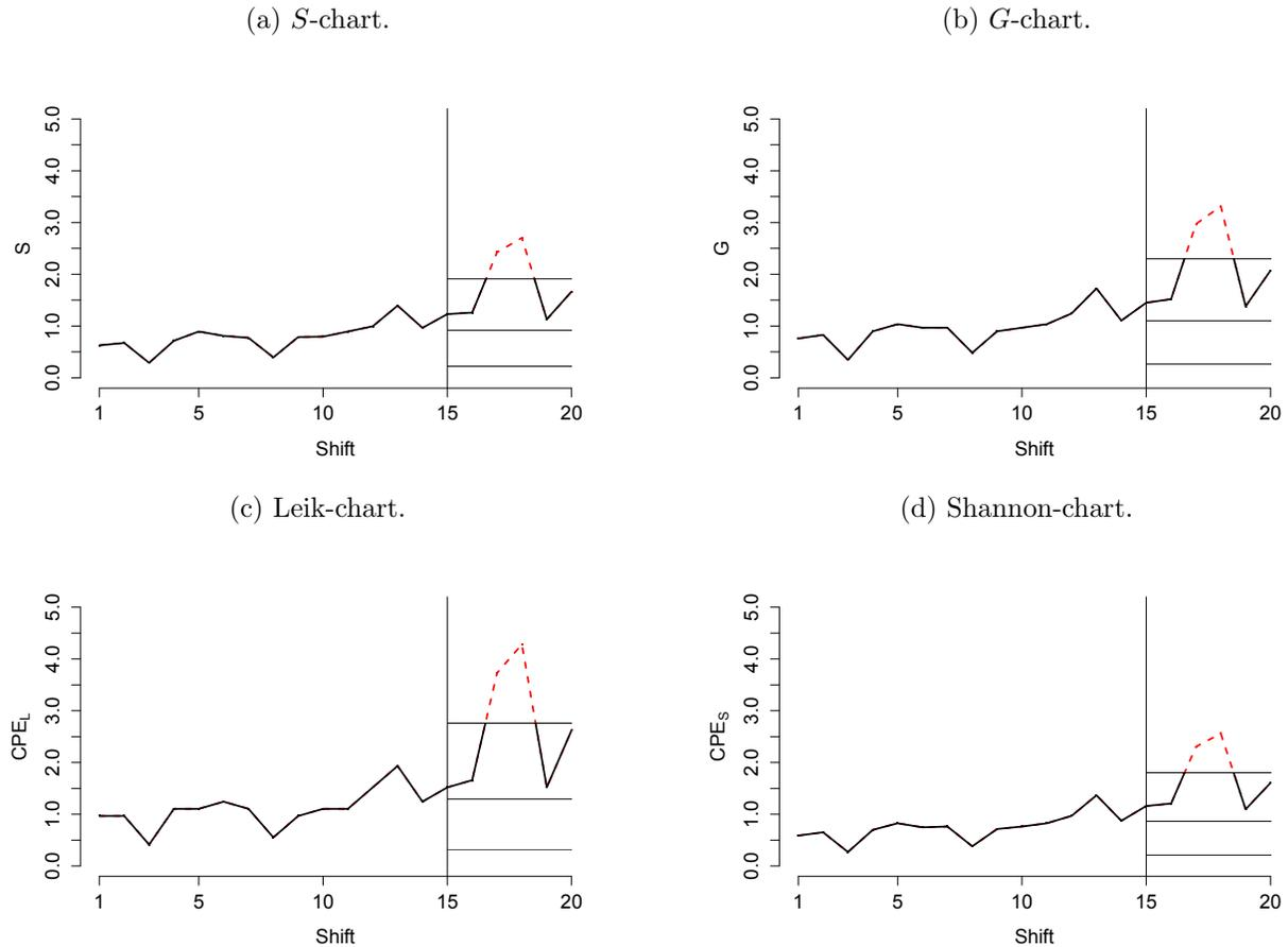
Figure 6:  $S$ -,  $G$ -, Leik-, and Shannon-chart of the data set from table 2. The first 15 shifts have been used to calibrate the control chart by estimating LCL and UCL. The charts are applied to the last 5 test shifts. Horizontal lines denote the UCL, the mean of the process, and LCL (top down). Red dashed line indicates an out-of-control situation.
