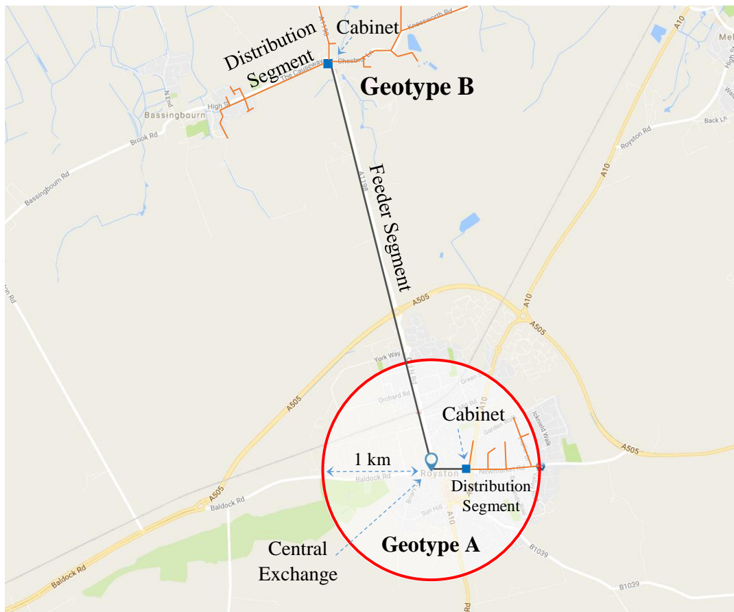
Figure 2 Examples of network elements in Geotype A and Geotype B emanating from the central telephone exchange in Royston, Hertfordshire, UK
