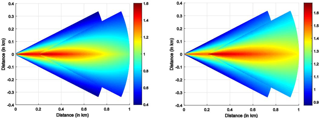
**Figure 5:** Simulation of wake effect with two consecutive turbines for an undisturbed wind speed of 7 m/s coming from the left, wind park A (left) and wind park B (right)
