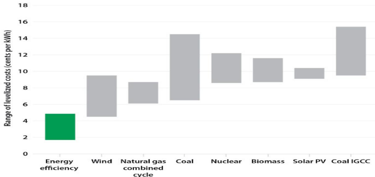
The high-end range of coal includes 90 percent carbon capture and compression. PV stands for photovoltaics. IGCC stands for integrated gasification combined cycle, a technology that converts coal into a synthesis gas and produces steam.
