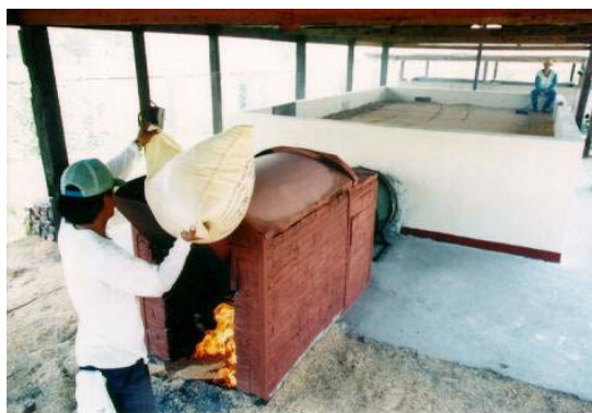
Fig. __. PhilRice adaptation of a high-capacity flatbed dryer from Vietnam models.
