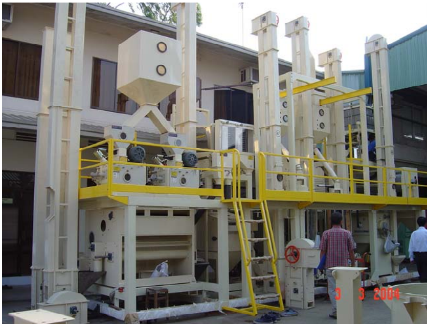
Fig. __. Modern rice mill systems employ multiple passes of grains through different mill components to maximize recovery and whole grains output.
