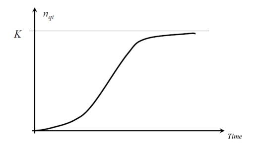
The simplest model that describes the path to S is the logistic equation where rq is the intrinsic
