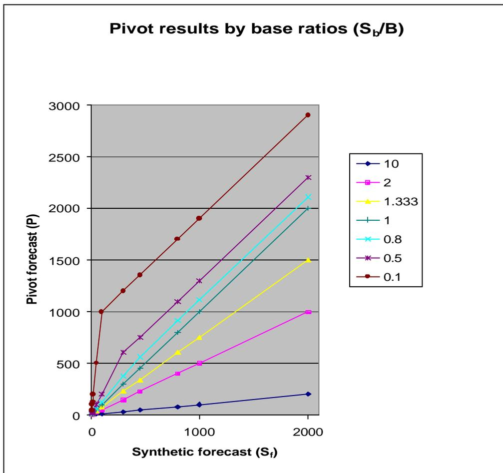
As is clear from this figure the results demonstrate that the switch from relative to absolute pivoting is applied when the ratio  $S_b/B$  is smaller than 1.0 and also that the switch point is applied earlier (with lower values for  $S_f$ ) when the ratio  $S_b/B$  gets much smaller than 1.0. This reflects the requirement to damp the predicted outcomes and to use more absolute pivoting when cells of these two matrices are less comparable to one another.
