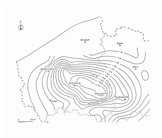
Fig 5 Height of rise of the deep ground water level
