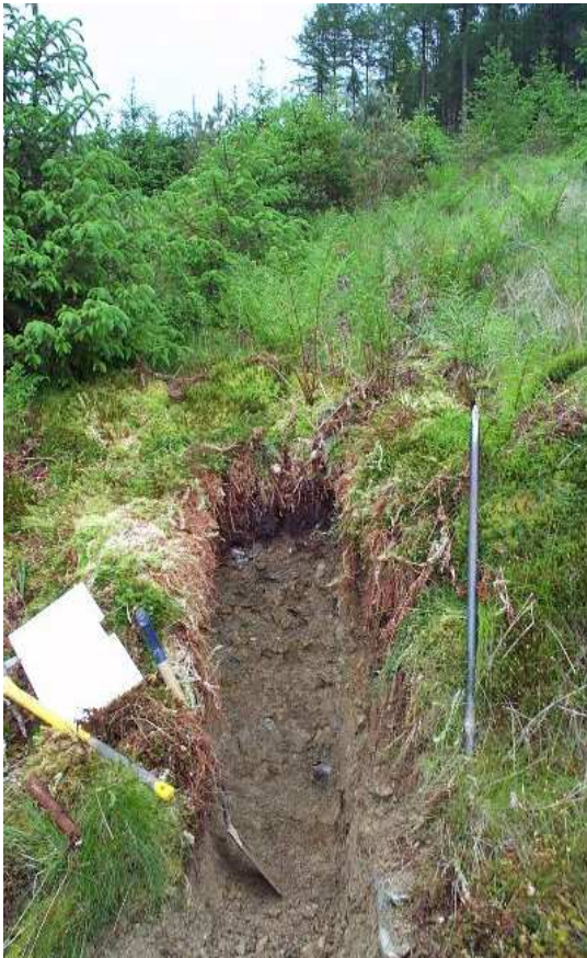
Figure 6(a) Site prepared for instrumentation, showing peat soil on glacial till
