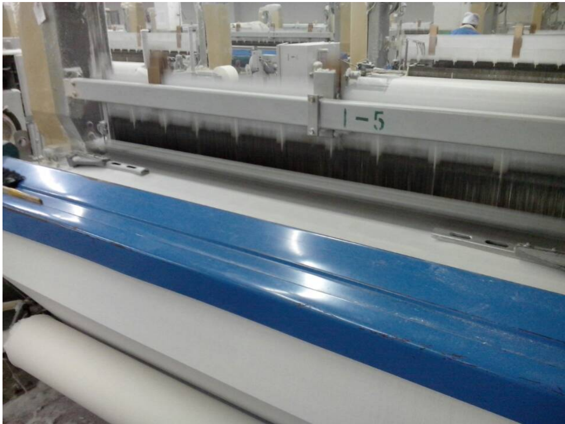
Figure A.4: Machine 5 (a Toyota air-jet loom), workstation 1
