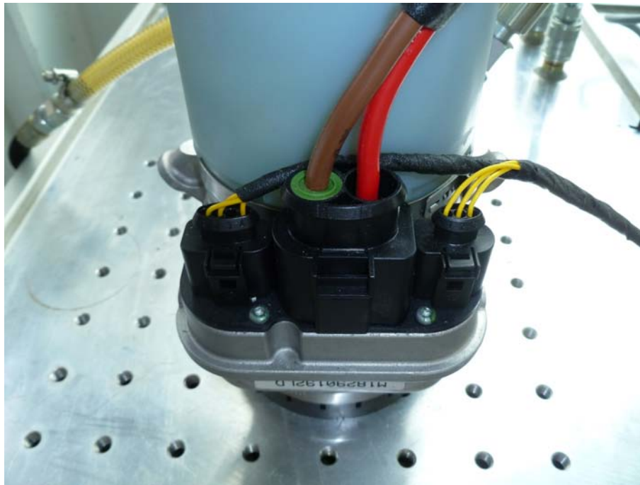
Figure 6 Pins of the EHPS of the VW Polo.
