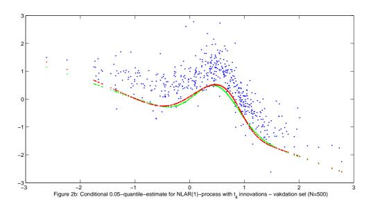
and the neural-network based quantile estimate  $q_n(x)$  (red curve). Mark that for pure autoregressive processes, the conditional quantile function is just a shifted version of the conditional mean m(x). Figure 1b shows the same picture for the data of the validation set. On the training set, we get an empirical level of 4.95%, i.e. a fraction of 0.0495 of the data  $Y_t$  are below the estimated conditional quantile  $q_n(Y_{t-1})$ . For the validation set, the empirical level is 5.61%.
