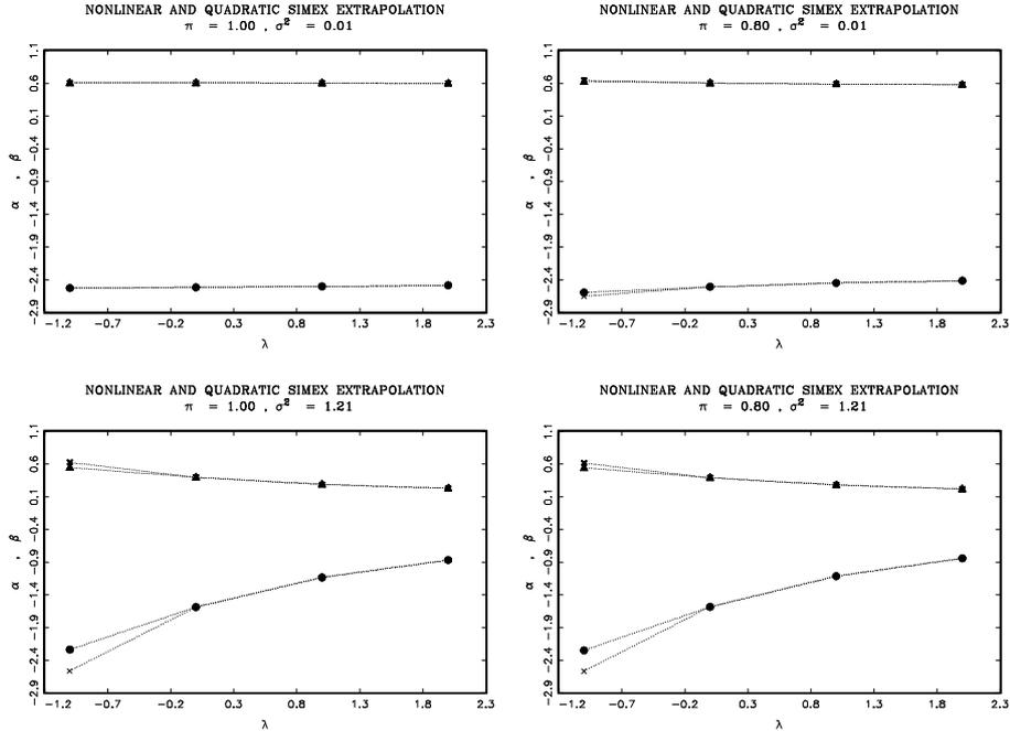
Figure 4/2: Nonlinear SIMEX extrapolation for different values of  $\pi$  and  $\sigma_e^2$ . ( $\blacktriangle$  shows estimates of  $\alpha = 0.60$  and  $\bullet$  those of  $\beta = -2.50$  in the quadratic case,  $\times$  indicates nonlinearly extrapolated values.)
